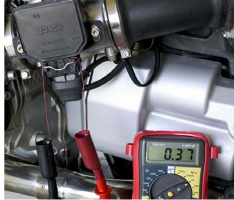
Figure 4: Probe wires inserted and plug reconnected
