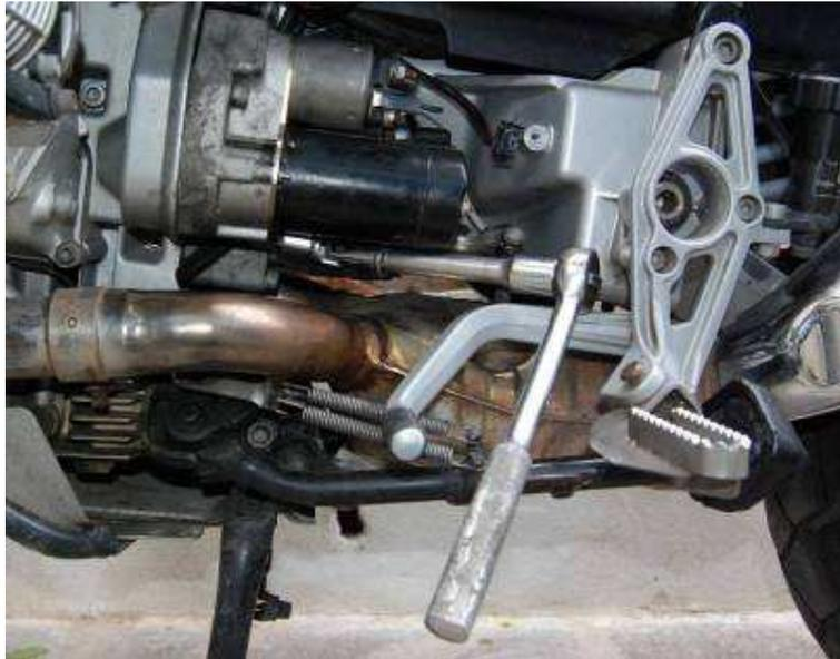
Attach the cable to the upper bolt and torque to 10 Nm, slide on the plastic-covered wire, attach the 12V auxiliary to the plastic cover and attach the screw to hold the plastic cover. Attach the battery cable and lower the tank, while being very careful with all cables and tubes. Do not forget to put back the bolt holding the tank.
