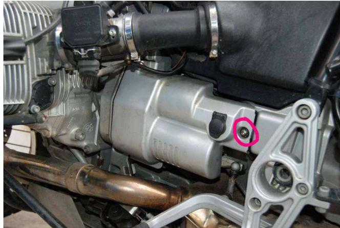
The starter is located behind a plastic shield found on the left-hand side of the bike. The cover is attached with a single T-25 Torx. After having removed the screw, move the cover slightly backward to disconnect the front. Detach the cable and remove the cover. What you will see is shown in the picture below.
