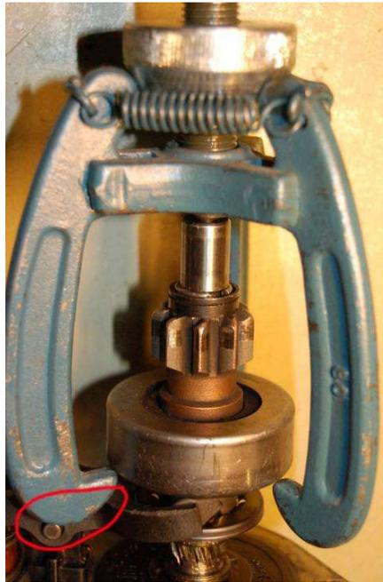
My puller (for the sake of completeness: The puller is the blue thing you see above) is slightly too large. If you look at detail inside the red ring, you will see that there is barely room for the puller between the starter gear and the lever. The problem is that the “arms” of the puller are too big. But I managed, and so will you (typical forward-looking statement).
