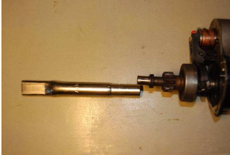
You hold the starter with the shaft pointing upwards, slide the extender down on the shaft so that it rests on the bushing. The pipe must not be too small – there must be some room between the shaft and the pipe (for reasons that will be apparent in a few moments). Carefully use a *small* hammer and tap the extender. The bushing didn't slide down? Well, tap it again using a little more force. After five wimpy tries, you'll give it a real knick, and off it comes! But be careful!
