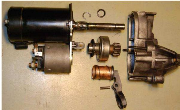
Now is the time to clean and grease. Look for any damages and excessive wear. The copper cylinder (it is called the solenoid) should not be greased, where it slides in. But clean it and make sure it slides properly.
