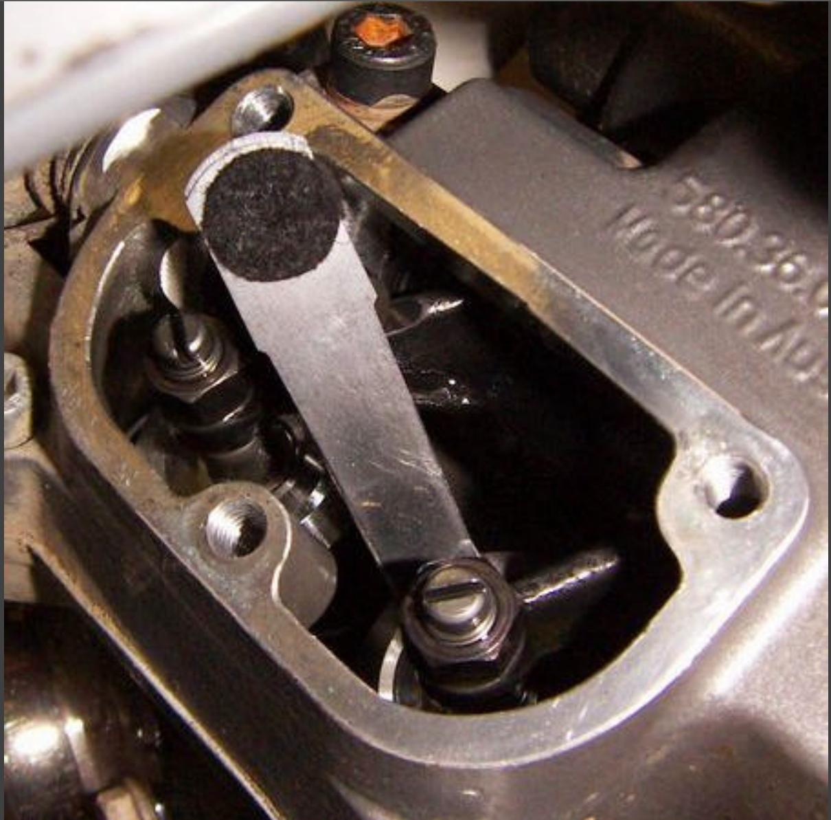
When you loosen the jam nuts, unless you have the previously mentioned  $\frac{1}{4}$ " drive torque wrench, you will want to note the effort required to do this as you will attempt to replicate the original torque value by feel. 🤖
