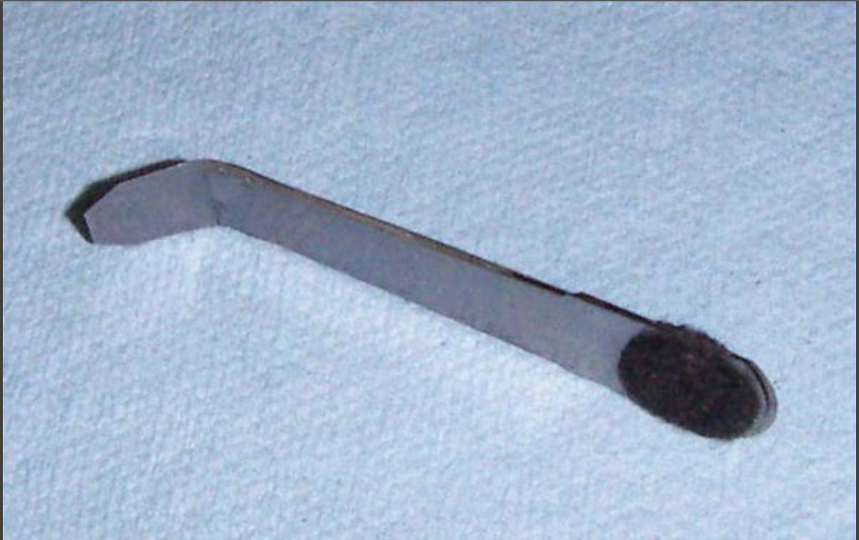
The idea is that with the space you have to work in being very "limited", the stiff handle offers more control and eliminates blade flex and bending... problems associated with a conventional feeler gauge blade.
