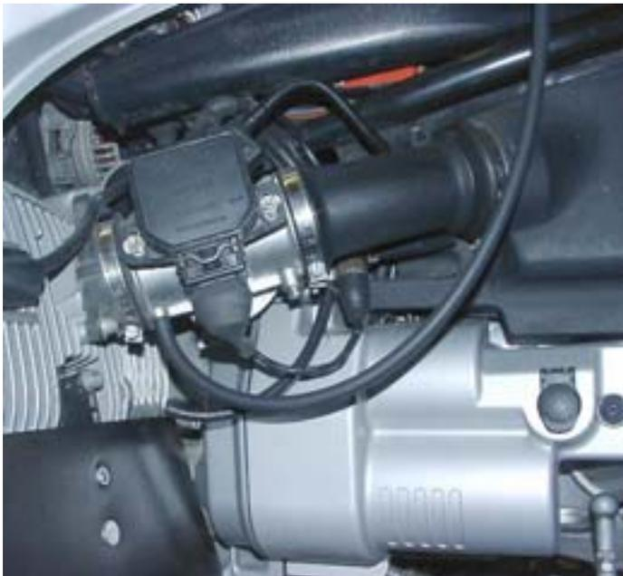
This works well during the initial setup but not during the On The Road Tests™©®QD. Why? Because you don't want the hoses interfering with your boots or the controls etc. During the On The Road Tests™©®QD I run the hoses down the tank, then slide the hose between the seat and the tank to help hold it in place then toward the TB's. Then I run it between the TB's, and the engine block, away from the throttle assembly, then a gentle bend back up to the intake air nipples.
