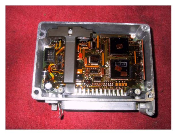
The eight pin connector mates with the hydro unit. It connects the two clutches and the two position sensors in the hydro unit. If you measure the resistance at the mating connector on the hydro unit, you can check the relative health of the clutches and position sensors.
