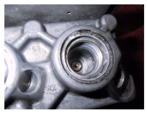
Now you are looking at the top of the piston. It has a little tit on the top that pushes up through the valve body you just removed and holds the ball bearing just barely off the seat when the piston is at the top, which is where it normally sits.
