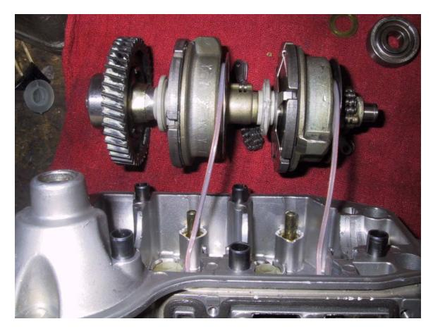
There is a couple of C-Clips on each end of the shaft. Take them off and the shaft components just slide off.
