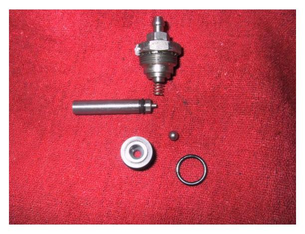
The front and back circuits are the same except that the piston for the front circuit is bigger.
