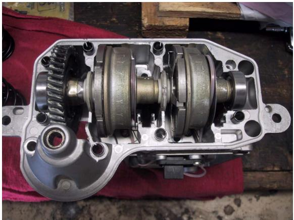
This picture shows the gear (motor is removed) and the two clutches.
