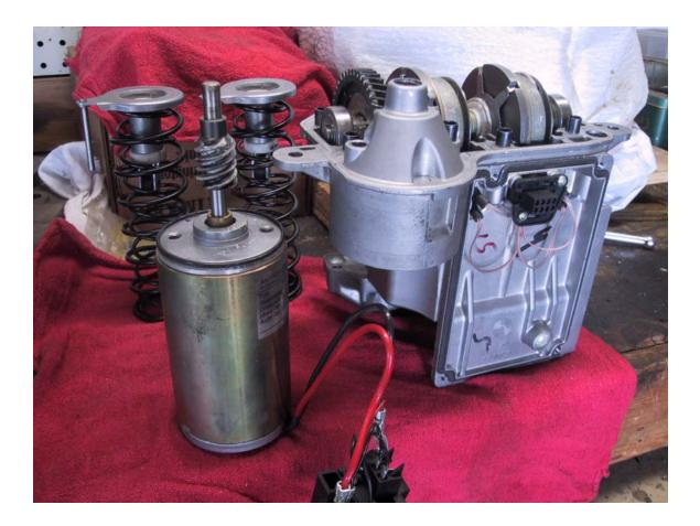
The motor is under a plastic cover. Also under the cover is the ABS relay and the connections that must be unscrewed to remove the ABS unit from the bike. The connections are under a cover that must be slid off. To slide it off, you have to push a sharp tool through the cover and depress a latch inside the plastic housing. Press a sharp tool (small screw driver or an awl or similar) right where there is a small circle above the FTW logo. You can see the hole I left in the picture below.
