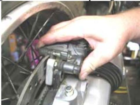
Gently try to lift the caliper assembly straight up. And, at some point you can **easily** lift the caliper assembly off the rotor and away from the bike. If it doesn't lift without friction, keep rocking the assembly until it does...
