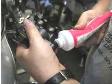
Lube the guides with the silicon grease. First the caliper guide...
