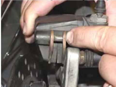
As the active pad makes contact with the rotor, the pistons continue pushing on the active pad – but, now, because the pad has made contact with the rotor, the pistons begin pushing the entire caliper assembly outward, away from the rotor. This is where the carrier guide pins come in - as the assembly continues to be pushed away from the rotor, it's riding on the carrier guide pins. (This bit here...)
