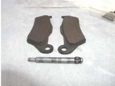
Notice the markings on the pin. That's scoring from the brake pads.
