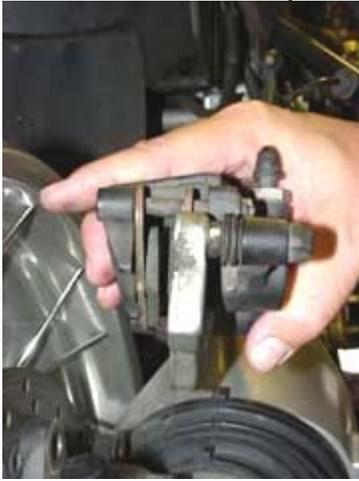
This slivery bit is the caliper carrier. This is the only bit that actually bolts to the bike. Everything else is free floating on this carrier.
