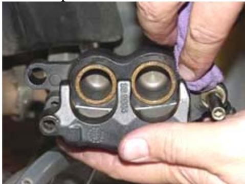
You're **NOT** going to stuff grease into every nook corner or cranny, or all over the edges of everything in sight – all you want is just a very light coating of copper anti-seize on the contact area between the pistons and the brake pads.
