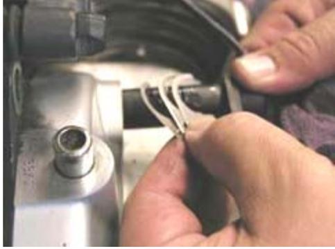
Get the bolt started by hand, then push the abs sensor the rest of the way in.
