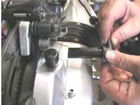
Gently rotate the ABS sensor clockwise and counter-clockwise (countre-clockwise) until it begins to insert. Work it in, rotating and wiggling, just like with the old lady, until there is only the last ¼ inch or so to go, then stop...
