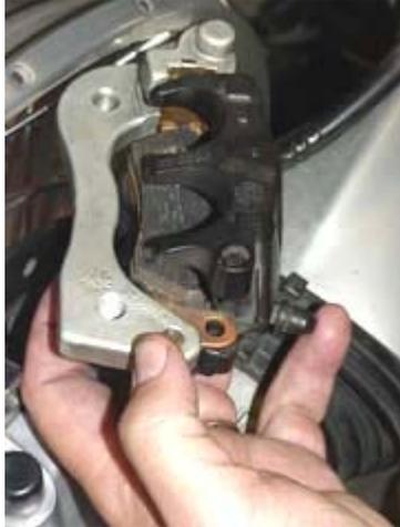
Insert the fixed pad in the caliper.
