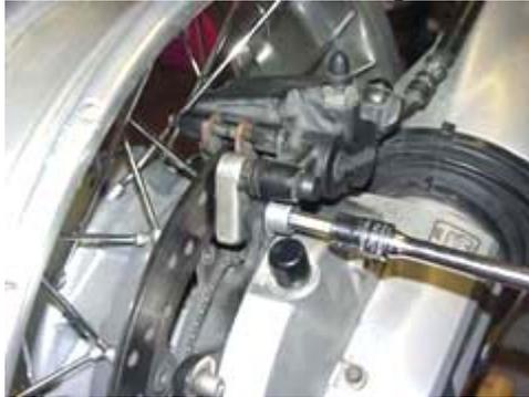
Then the front bolt...It has the ABS cable anchor plate that also serves as a washer
