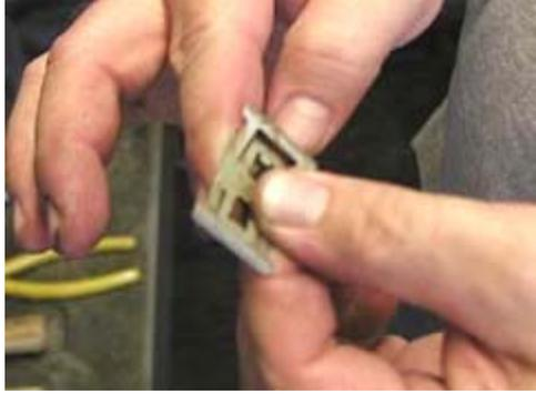
This little clip sits up inside the brake caliper and on ‘top’ of the pads and applies downward pressure on the pads. This keeps the pads from rattling, or chattering, in the caliper assembly when the pads are both engaged and resting free. Let’s make sure there are no oddities in the clip – check to see if it’s broken, if tabs are sheared or especially if it has noticeable wear anywhere.
