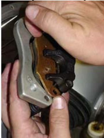
Align the heel pad to the heel pad base clip. Then drop in...
