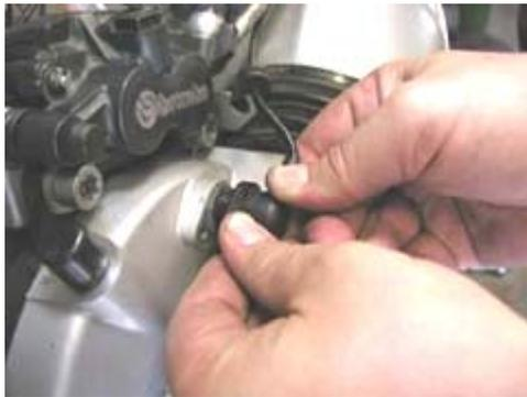
So you can insert the shims and put anti-seize on the ABS sensor bolt.
