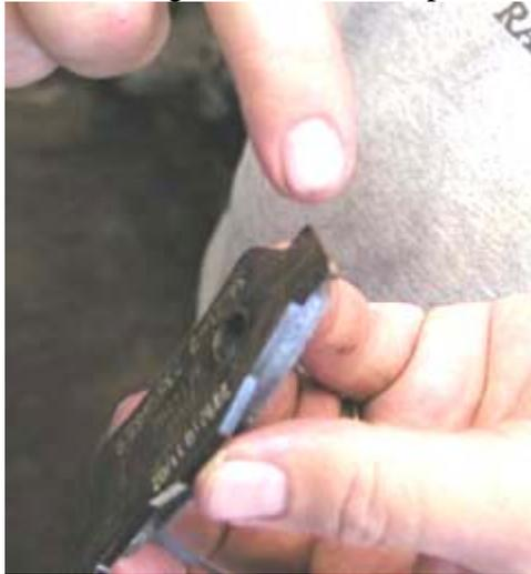
Wipe off the excess anti-seize from the edges of the pads
