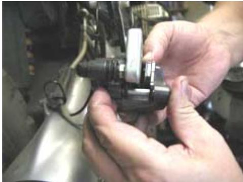
Give the head of the pin a light tap or two with the mallet to seat the pin.
