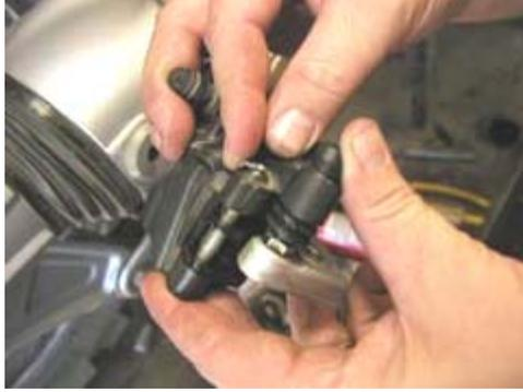
Put circlip back on.
