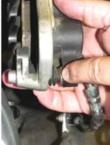
Now carefully rotate the carrier in space so you can look at the brake pad's 'heel'..
