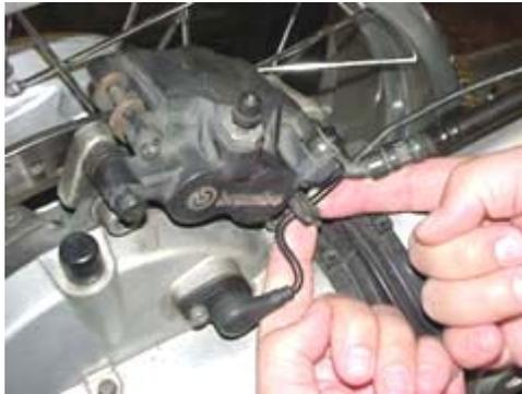
Next, you'll pull the ABS sensor, because you're gonna be waving that whole brake assembly around in the air in a minute...
