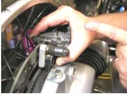
Then reverse the motion and tilt the brake assembly back the other way... Here we're pushing in with the thumb and pulling towards us with the fingers.
