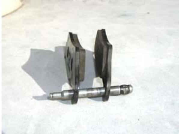
The pin incurs a lot of the braking force when the pads are engaged, and there is a fair amount of sliding force across the pin as the pads are engaged, and released. The wear occurs in different places as the pads are consumed. A lot of wear on this pin can influence brake wear, and it may indicate other problems.
