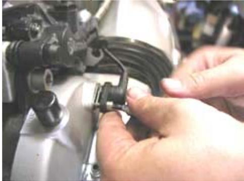
Tighten with a sneerk. Put the rubber grommet (and ABS sensor cable) into the holder and secure the ABS sensor cable to the hydraulic hose with one or two ty-rap(s)
