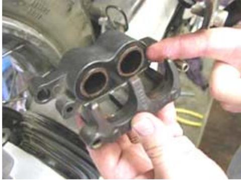
You are going to put just the finest sheen of copper anti-seize grease on the pressing surface of those pistons...
