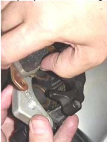
Align the heel of the pad to the heel pad base clip. Then drop the pin side of the pad, then push the pad in so that it rests on the caliper pistons. You may find that it helps to slide the carrier ‘back’ to allow more room for the pad to drop onto the pistons.
