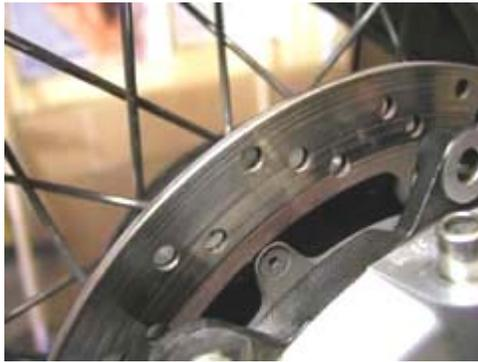
On this rotor, at 23,000 miles, there is no significant scoring, so this disc is in fine shape - we'll just move right along.
