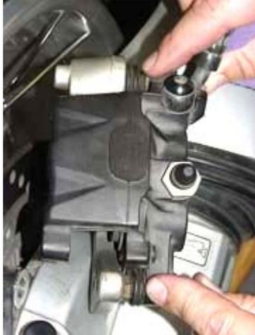
These gaiters protect the carrier guide pins from accumulation of spooge.
