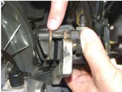
Note how it rests against the backside of the brake caliper assembly. That's why we say it is 'fixed' in place. This pad doesn't move much, in fact it shouldn't move at all (with respect to the caliper assembly). It is simply pulled onto the rotor as the 'active' pad is pushed into the rotor by the pistons.. Sounds easy, huh?
