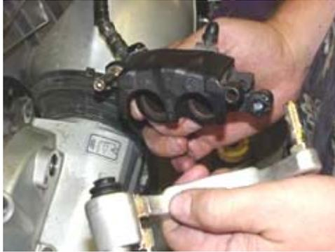
And gently align the caliper and carrier together...
