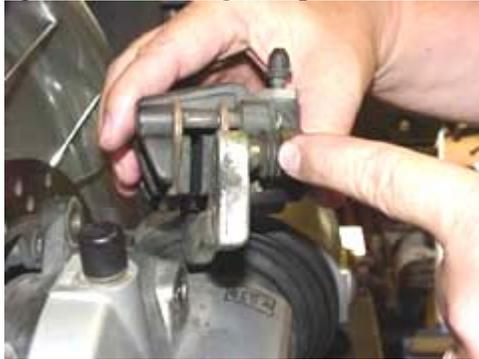
As the pushing continues, the pad on the backside gets pulled toward, and eventually makes contact with, the rotor, et voila – both pads are engaged – and, slowing ensues. And here is where it is so weird that Javarilla freaks everytime he thinks about it – nothing supplying the slow is bolted to the bike. It's all just slidin' around like an excited dog on linoleum on those carrier pins.
