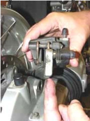
This is one of the caliper carrier guide pins – it's under the rubber gaiter...
