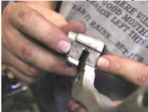
This is an interesting little piece, here. This is where the heel of the brake pad sits. When you're braking, tremendous force is projected into this little surface. Not only that, but this surface also incurs some lateral movement as the pads squeeze and retreat from the rotor. We want to treat this little guy with the respect he deserves.
