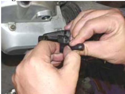
Until you can pull the accordion end of the gaiter through to the other side, leaving only the knob exposed. Take joy in this. It's one of the few times you can leave your knob exposed on purpose.
