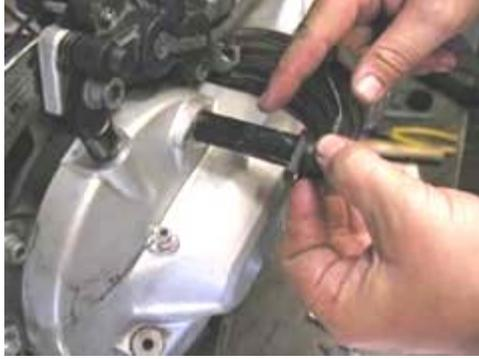
Insert the ABS sensor into the final drive.
