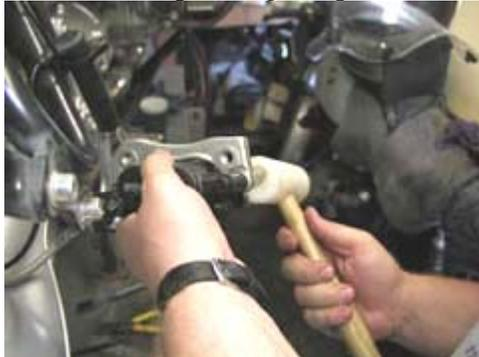
Slide the clip onto the end of the pin's groove – shoulder side in... If the groove of the pin doesn't 'stick out' far enough for the clip then the pin hasn't fully seated yet.
